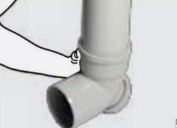
DURABLE SOLFIT Pipes and Fittings are joined with the help of DURABLE SWR Solvent Cement, which is a single step fast setting solvent cement. The bonding takes place due to chemical fusion of the mating surfaces.
