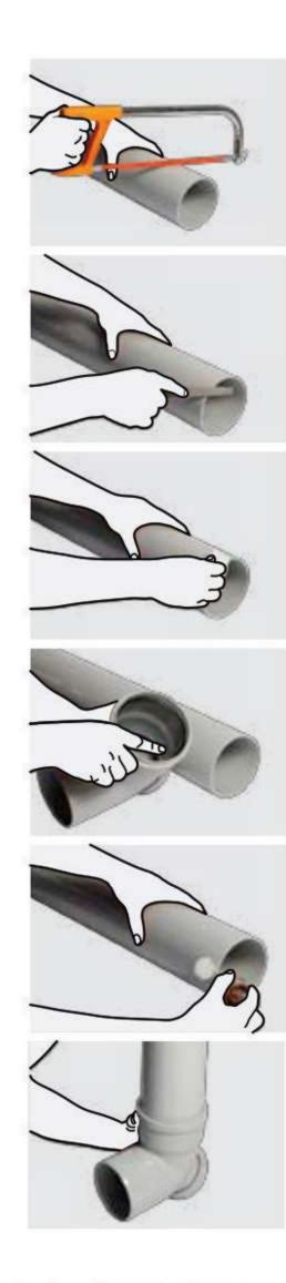
DURABLE RINGFIT Pipes and Fittings are joined with the help of DURABLE SWR Lubricant. For faster plumbing and leak proof joints we strongly recommend the use of DURABLE lubricants only.
